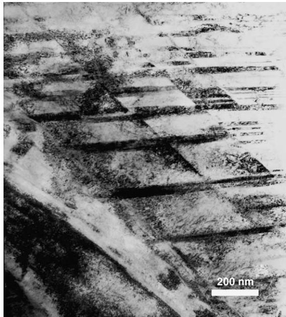
Fig. 11. Bright-field images shows intersections of two sets of twins at 3 dpa with irradiation and test temperatures of 44 and 50 °C, respectively.
